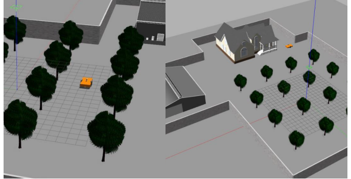
Fig. 6: Gazebo simulation showing the robotic platform inside a mockup virtual orchard
