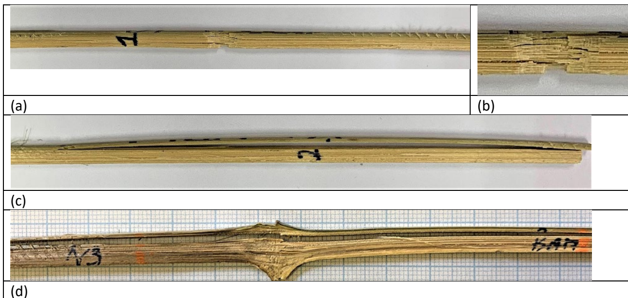
Figure 18. Two typical failure mode: (a) a defibring in the middle zone zoomed in (b) and a delamination of the cortical layer, in an internode (c) and with Node sample (d).
