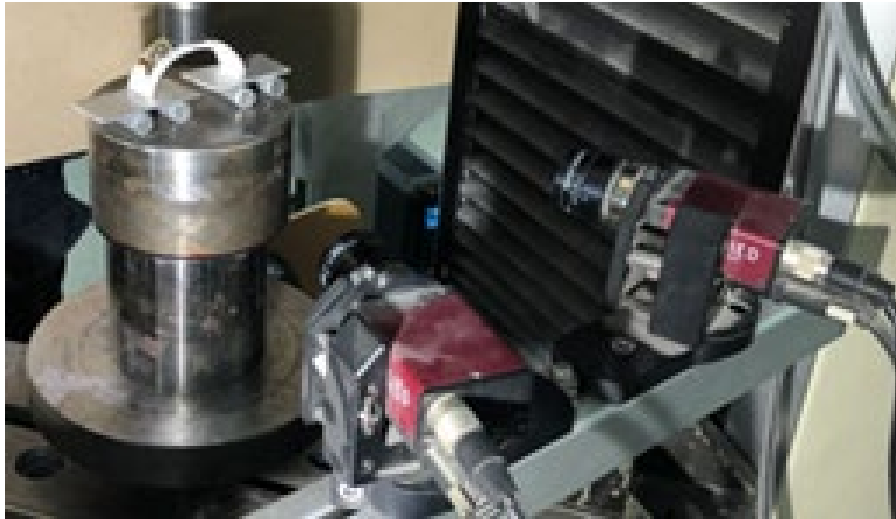
Figure 3. The set up for the semi-ring test with DIC
