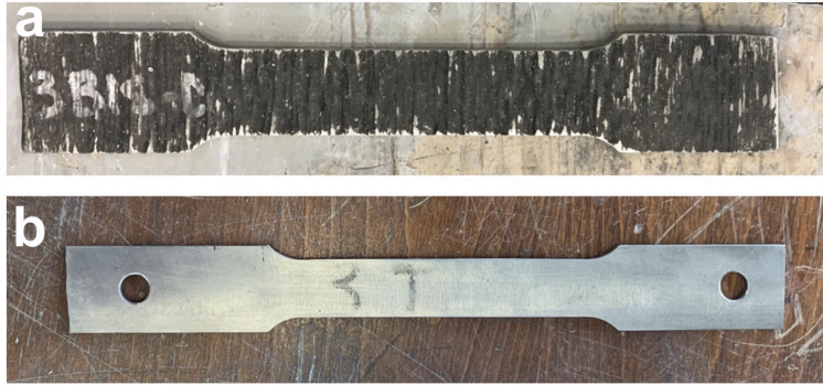
Figure 2: Tensile specimen cut from WAAM plates: (a) as-printed and (b) after surface milling.
