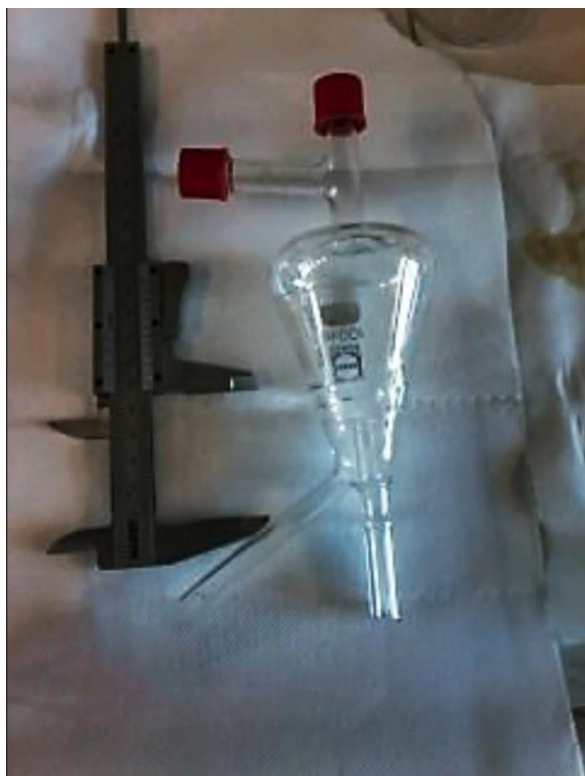
Figure S2. Picture of the 100 mL vapor condenser.
