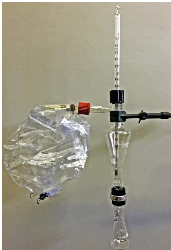
Figure S1. Picture of the 25 mL reflux condenser.
