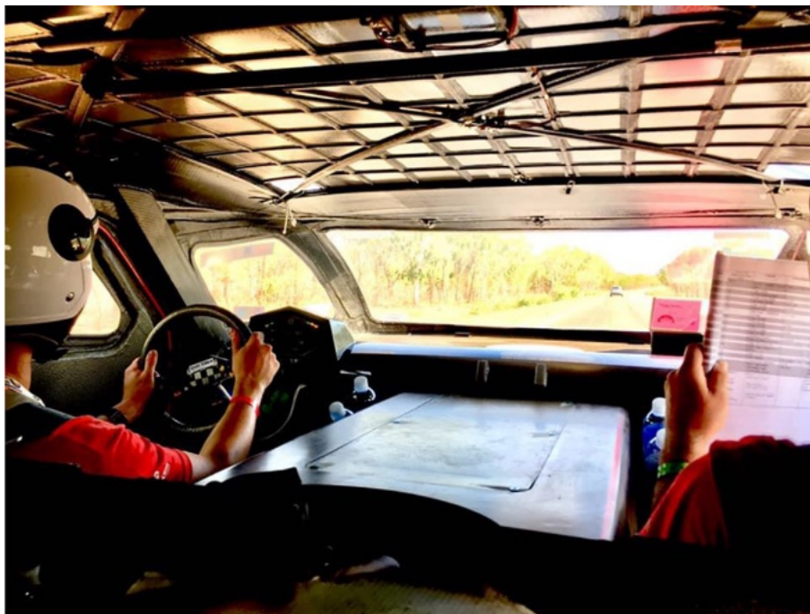
Fig. 23. Vehicle interior after design changes. The new composite structure eliminates all vertical metal bars inside the cockpit improving drivability and usability.
