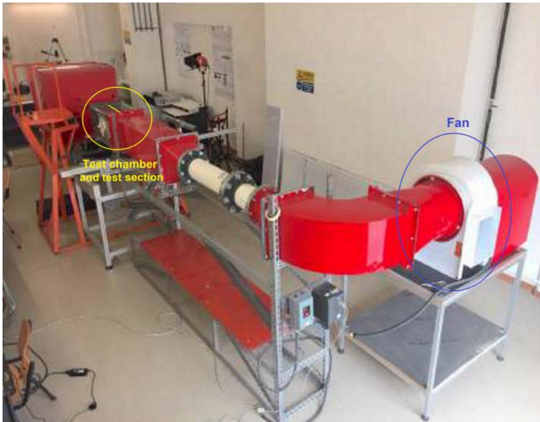
Figure 2: Picture of the entire wind tunnel at the Department of Industrial engineering (DIN). The test chamber and the test section have been highlighted in yellow and the fan have been highlighted in blue
