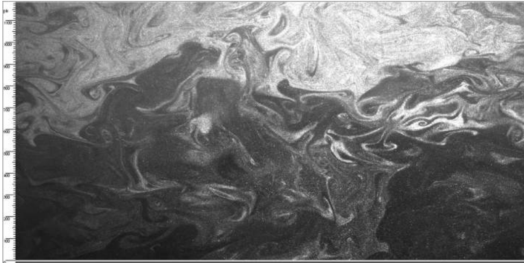
Figure 9: Example of a picture watchable in a PIV experiments. In specific, this is obtained during the test conducted with the sample of screen H5.
