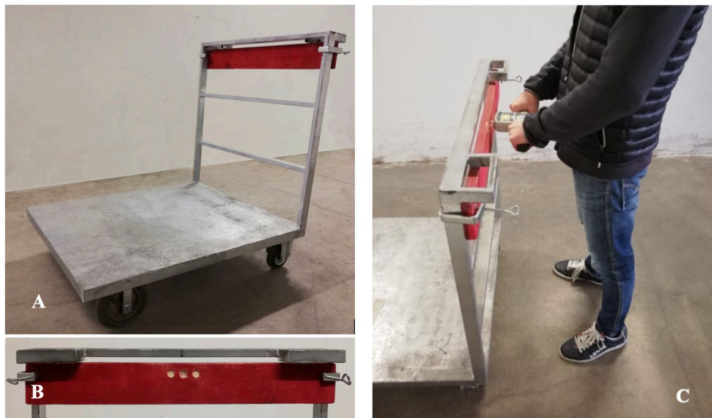
Figure 1-A, 1-B and 1-C. Industrial trolley adopted in the study (A), flat adaptor on the trolley handle (B) and force gauge in position (C).
