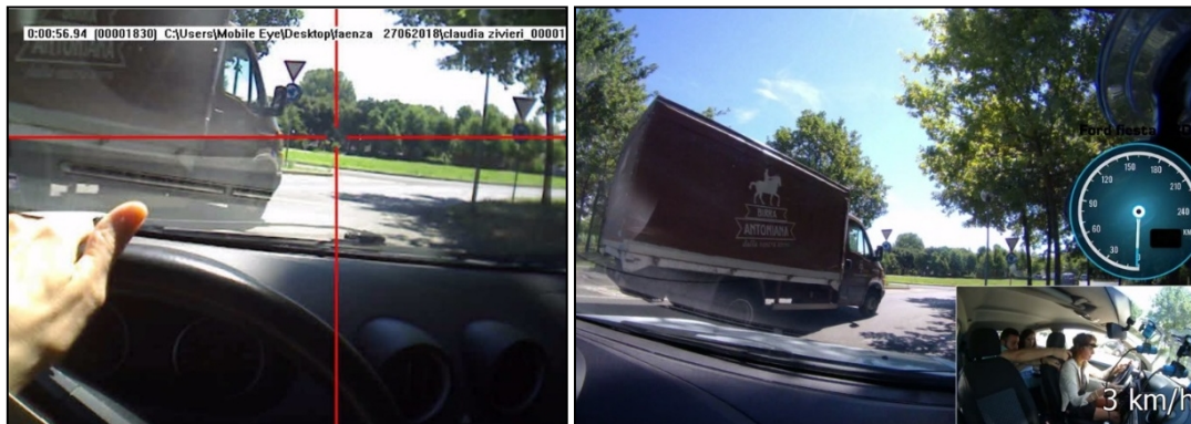
330 331 Figure 5. Synchronization of the ASL eye-tracking mobile video output with the VBOX PRO video output. 332 333
