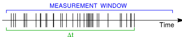
FIG. 5. A saturating buffer in an FPGA will show, at the end of the recording, a buffer whose end is devoid of events. We therefore choose the observation time \Delta t to be the portion of the buffer ranging up until the last observed event in order to prevent incorrect assessments due to saturation.
