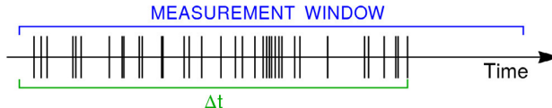
FIG. 5. A saturating buffer in an FPGA will show, at the end of the recording, a buffer whose end is devoid of events. We therefore choose the observation time \Delta t to be the portion of the buffer ranging up until the last observed event in order to prevent incorrect assessments due to saturation.
