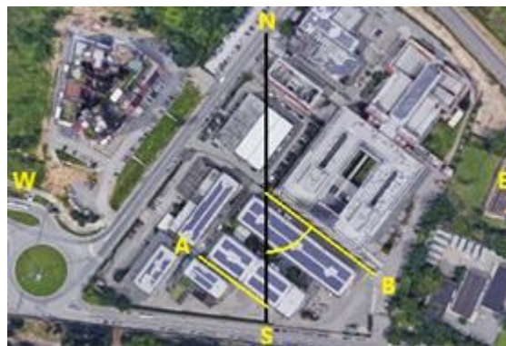
Figure 30 Map of the two street canyons (A: painted canyon; B: reference canyon) in the Lazzaretto area (Bologna, Italy) with indication of the N-S orientation (source: Google Maps).
