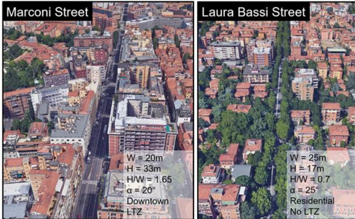
Figure 15 Street views and details ( W = width, H = height, \alpha = orientation angle of the street canyon) of the two street canyons in Bologna (source: Google Earth).
