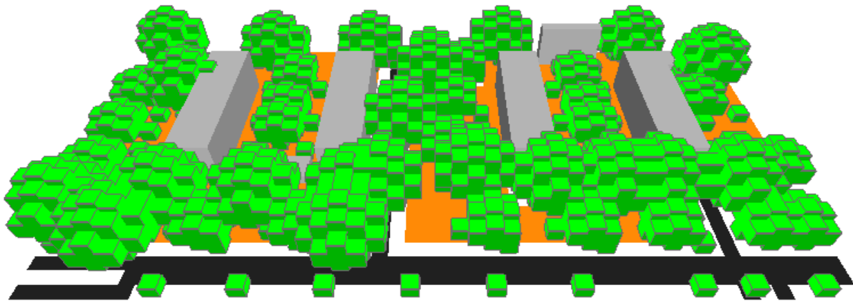
Figure 25 A 3-dimensional picture from the ENVI-met tool 'SPACE' of the Myyrmäki Vaskivuorentie area; gray: buildings, light green: trees with different heights and shading areas, orange: unsealed loamy area, not vegetated; white: sealed areas, stone slabs, black: main sealed roads with tarmac. Adapted from D5.3.
