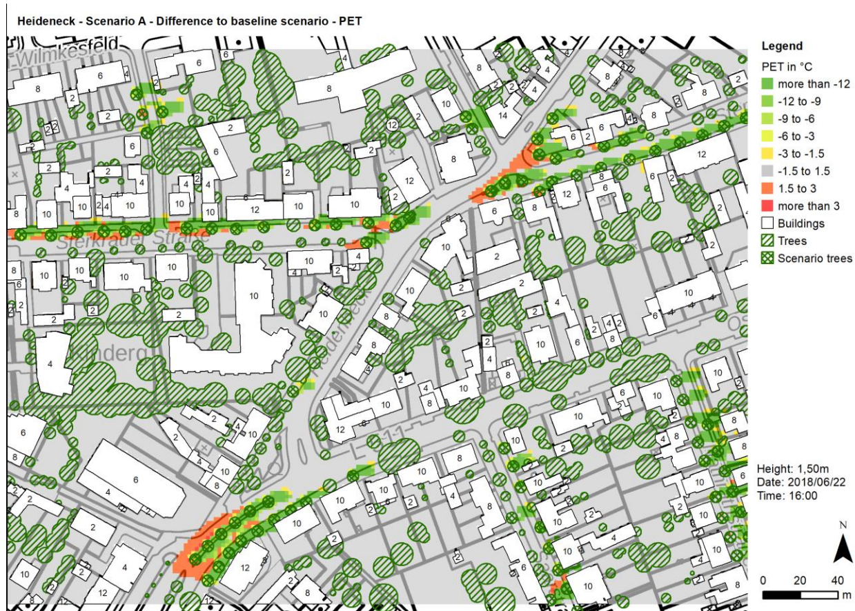
Figure 37 Model Bottrop 1 (Heideneck): Scenario A – Difference of PET values, scenario A minus baseline scenario (source: own account, data: City of Bottrop)
