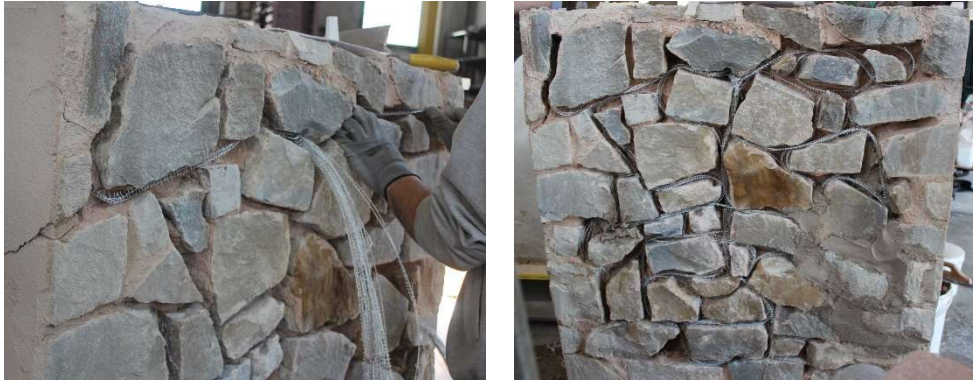
Figure 4. Reinforcing procedure for the sample S_I-MA_B200-S600, Reticolatus technique.
