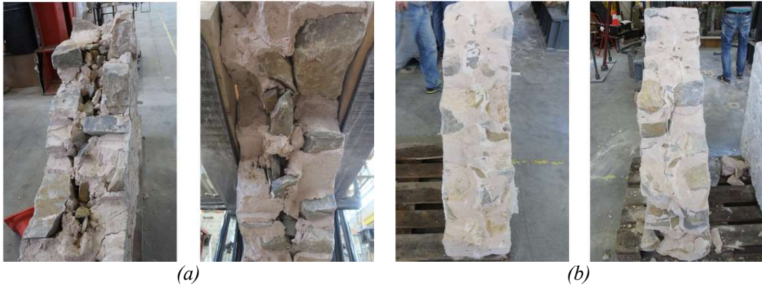
Figure 13. Detail of the cross section of the samples after the tests: (a) sample S_I; (b) sample S_I-MA.
