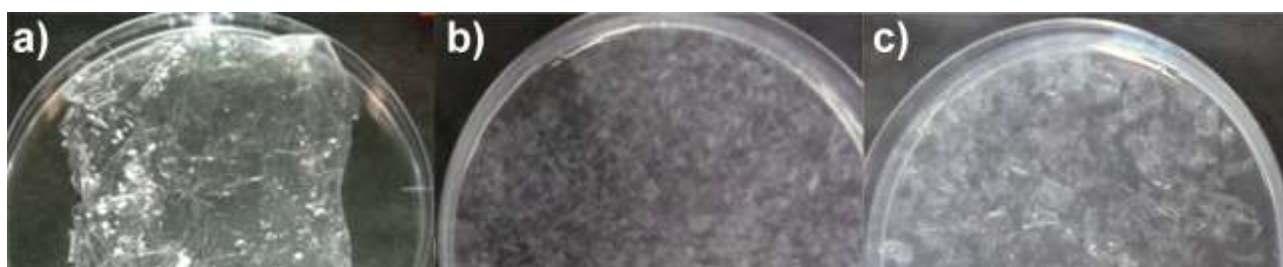
Figure 3. PVC films incubated in the abiotic control (a) and in the presence of P. citronellolis (b) or B. flexus (c) for 70 days. Data from experiments performed in duplicate.
