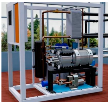
Figure 1. StarEngine micro-ORC installation at the well site
