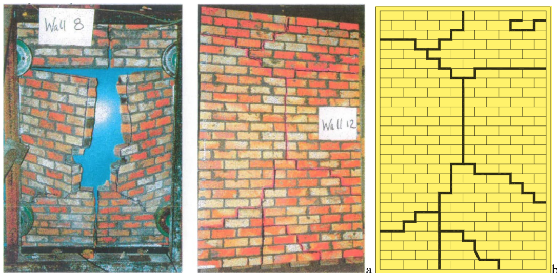
Fig. 13 – Experimental crack pattern: a) photos of the failure of Wall 8 and Wall 12 from [53] and b) sketch of the crack pattern of Wall 12.
