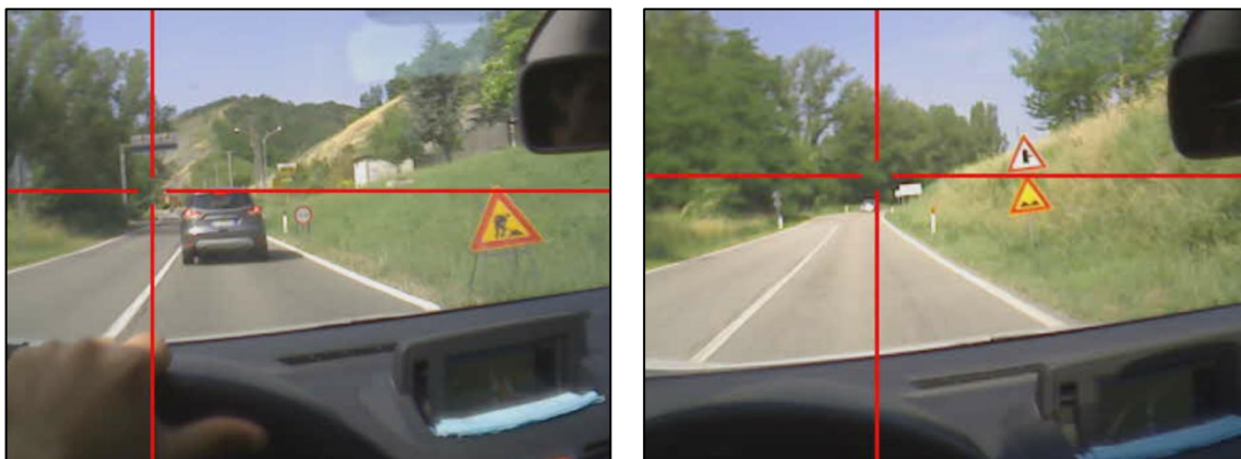
186 Figure 1: Tripod-mounted temporary sign (left) and pole mounted temporary sign (right). All 187 temporary signs were triangular in shape, with a yellow background and a red border.
