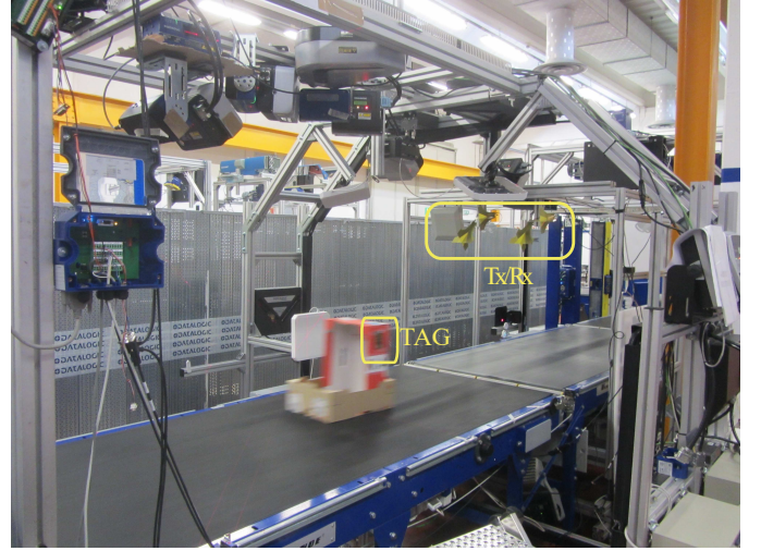
Fig. 4. Luggage sorting on a conveyor belt using UWB-RFID tags [25].
