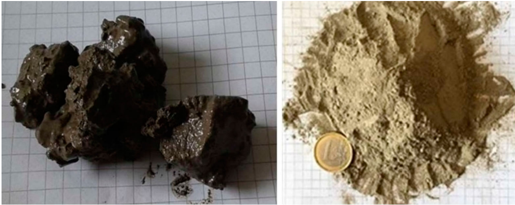
Figure 3. GP before and after drying process.
