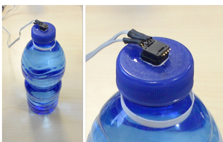
Fig. 5: The sensorized graspable object (left) and detail of the pressure sensor (right).
