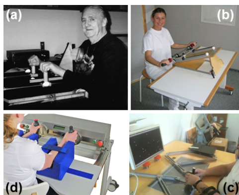
Fig. 1: Existing bimanual training systems: (a) Batrac [13] (b) Nudelholz [21] (c) Bimanual Haptic Desktop [23] (d) Bi-manu track [22]
