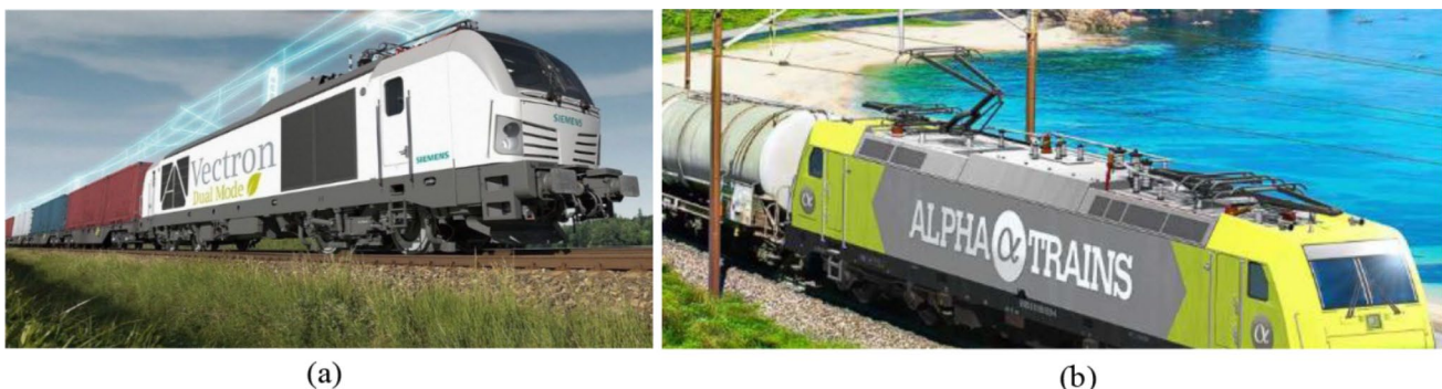
Fig. 6 Latest freight trains (a) Vectron Dual-Mode Locomotive (Source: SIEMENS [86]), (b) Alpha Trains Hydrogen Locomotive (Source: Alpha Trains [66])
