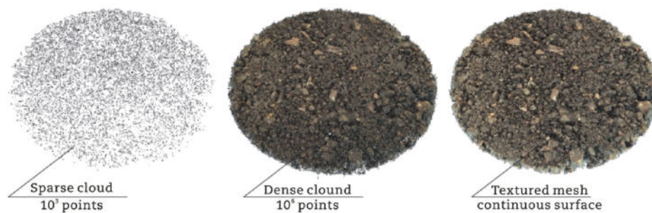
Fig. 3 – Close-range photogrammetry 3D-model generation.
