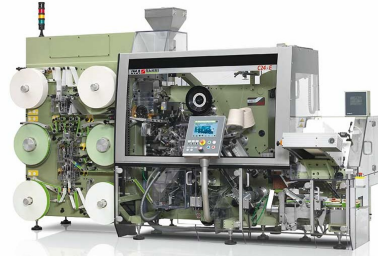
(a) The local storage wagon. 1 is the filter-paper reel, 2 is the tag reel, 3 is the outer-envelope reel, and 4 is the VL-shaped marker.
