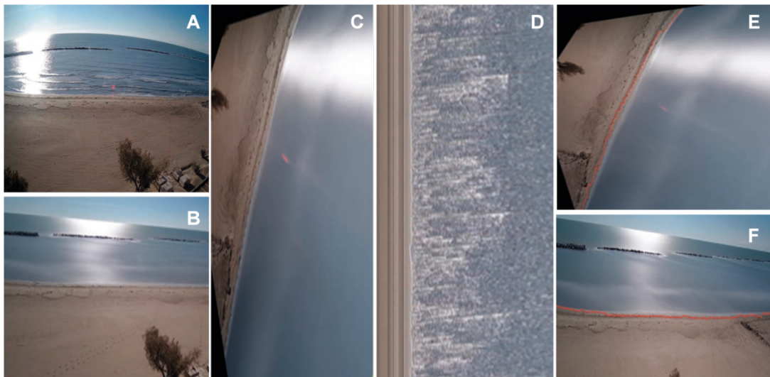
Figure 5. Example of SNAPSHOT (A), TIMEX (B), RECTM (C), TIMESTACKS (D), RECSH (E) and TMXSH (F) for the Riccione site.
