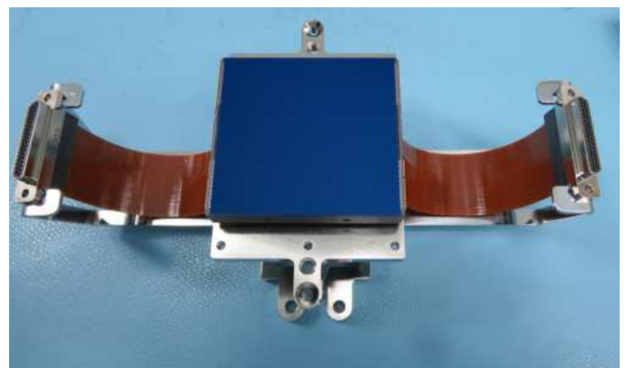
Fig. 8. CCD273-84 developed specifically for VIS by e2v Technologies.
