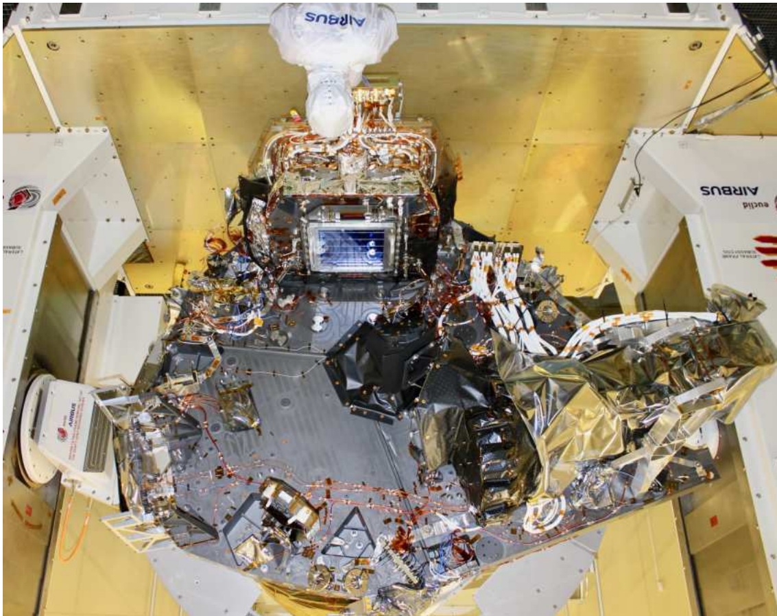
Fig. 5. Disposition of the VIS Focal Plane Array on the Payload Module baseplate. In this image, which is in the same orientation as Fig. 4, the detector array is visible under a protective transparent cover, as the hood is not yet in place. The Shutter and the Calibration Unit are not yet integrated. Image courtesy of Airbus.
