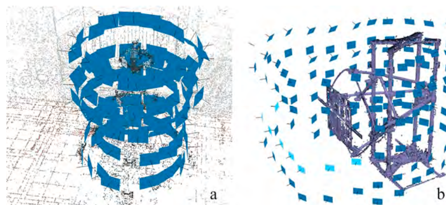
Figure 17. Radial camera network for the horizontal (a) and vertical (b) repro stands.
