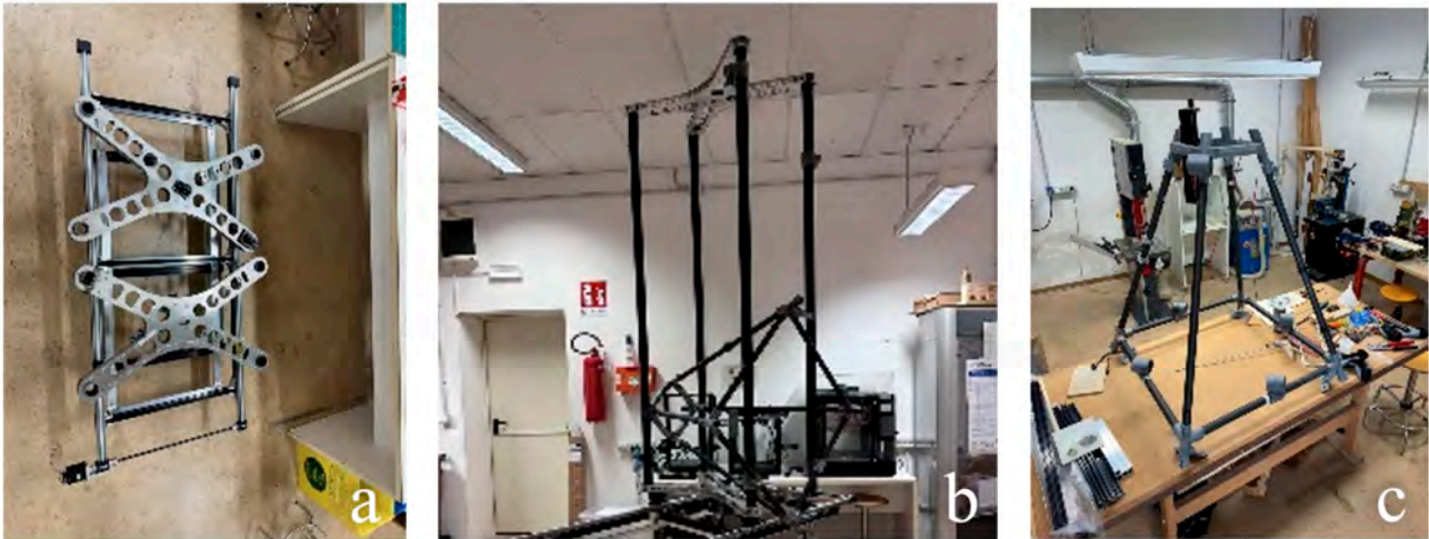
Figure 6. The elements of the vertical stand main structure: lower frame (a), vertical frame (b), and trapezoidal frame (c).
