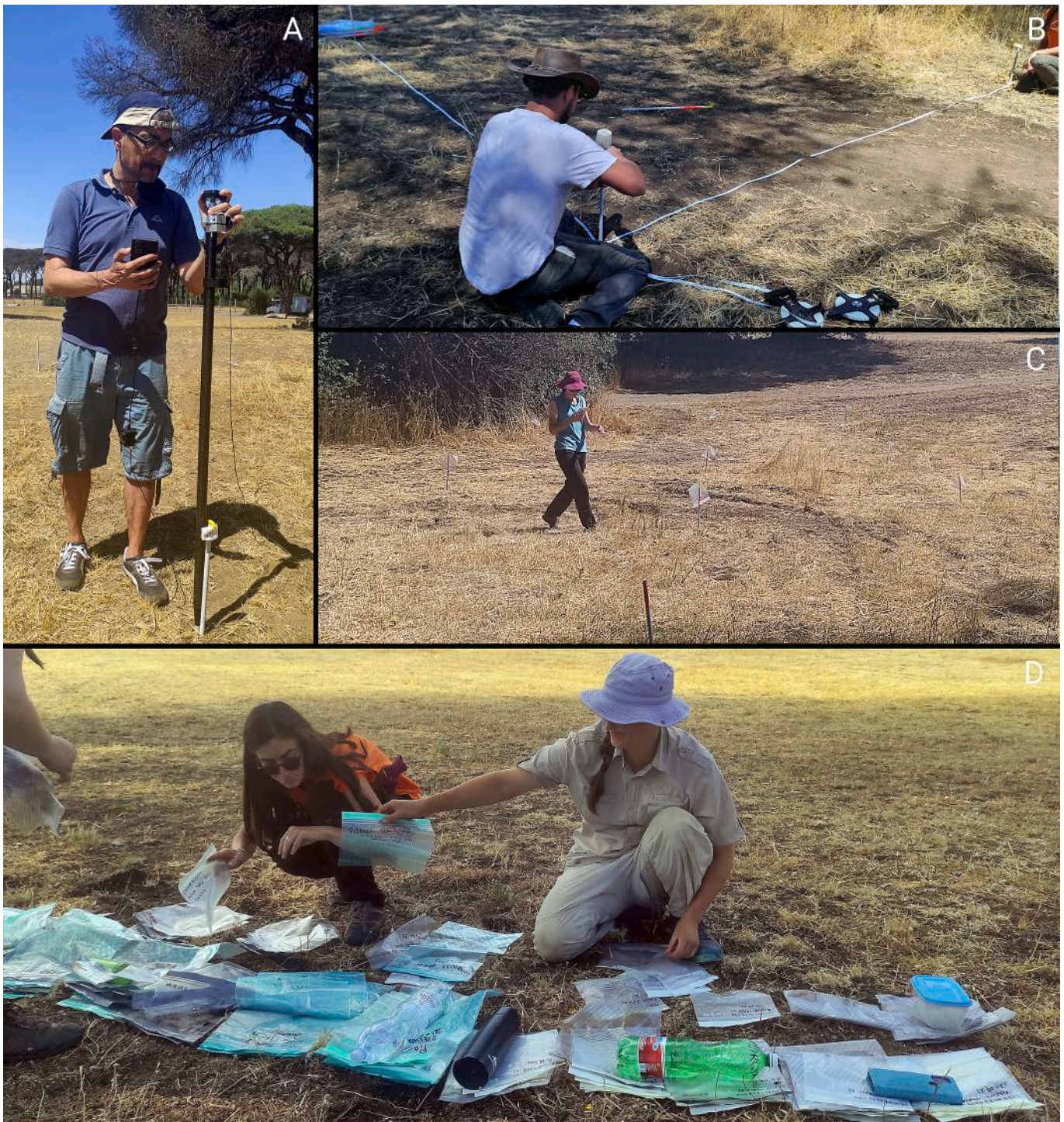
Fig. 6. Different steps of the survey. A, placing the sticks with the low-cost device. The survey pole turned out later not to be essential. B, placing the intermediate sticks with the measuring tapes. C, plastic bags to collect the materials with the name of the site, the name of the unit (coordinates of the stick) and the data were immediately placed over the sticks. So, we could recognise if a unit had already been surveyed by the presence/absence of the bag. After surveying the unit, walkers had to upload the ancillary data on Epicollect with their smartphones. D, at the end of the day, a matching control between the Epicollect entries and the bags was always performed.
