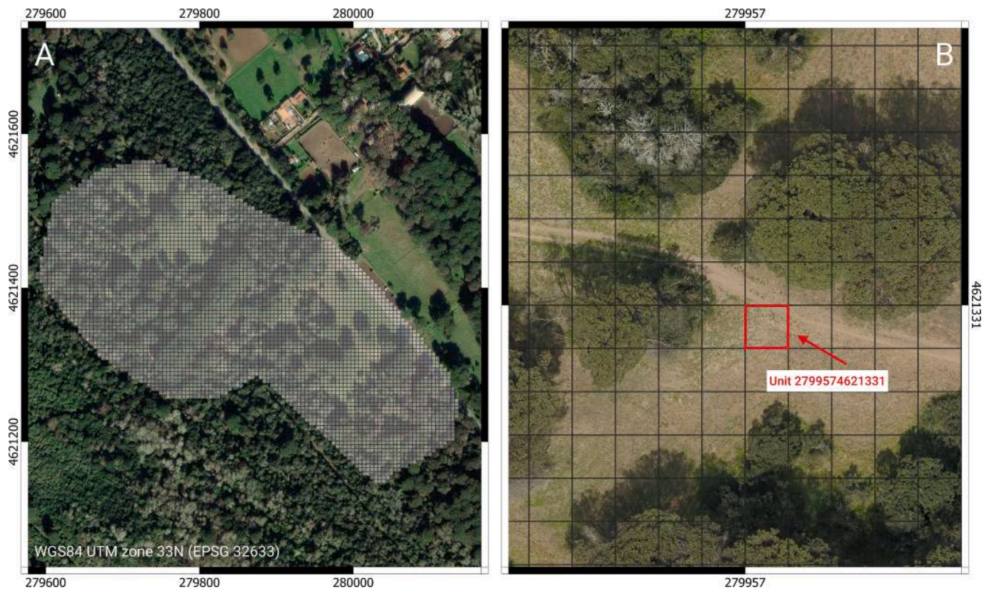
Fig. 5. A, the established grid, based on WGS84 UTM zone 33 N (EPSG 32633), background ESRI satellite imagery (Esri, DigitalGlobe, GeoEye, i-cubed, USDA FSA, USGS, AEX, Getmapping, Aerogrid, IGN, IGP, swisstopo, and the GIS User Community). B, the procedure to assign the name to every single unit, background aerial image from our drone flight.
