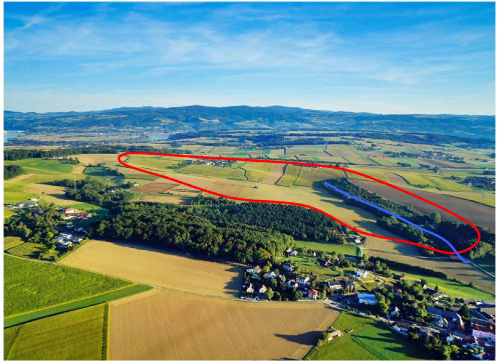
FIGURE 1 Aerial photograph of the 66 ha Hydrological Open Air Laboratory (HOAL) in lower Austria. Red line indicates the topographic catchment boundary, blue line indicates the main stream of the catchment. Photo: A. Eder
