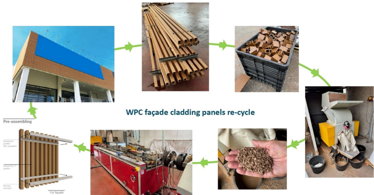
Fig. 12 WPC façade cladding panels: an example of the re-use cycle, from Novowood ®
