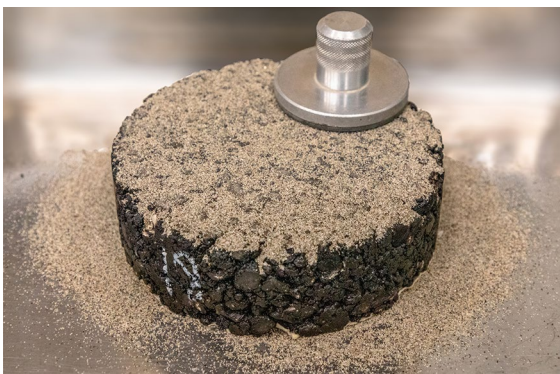
Fig. 5 Performing the Volumetric Patch Test
