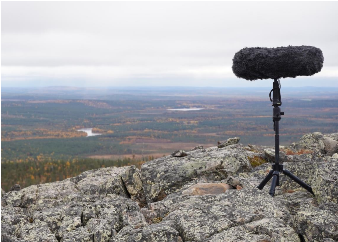
Figure 11 Omnidirectional stereo (A-B) field recording setup at Leviduottar, Levi (Renzi 2022).
