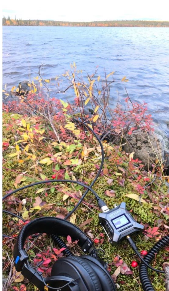
Figure 13 Recording wind-water interactions with hydrophone at Bállásjávri, Muoná (Renzi 2022).
