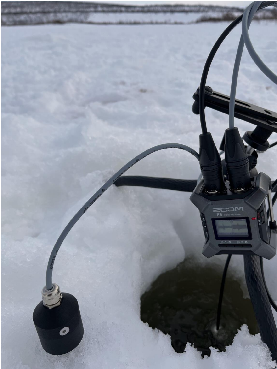
Figure 41 Fishing sounds in Suoidnesuolu, Guovdageaidnu, with a geophonic sensor spiked in the ice and an hydrophone dropped inside an ice-fishing hole (Renzi 2023).
