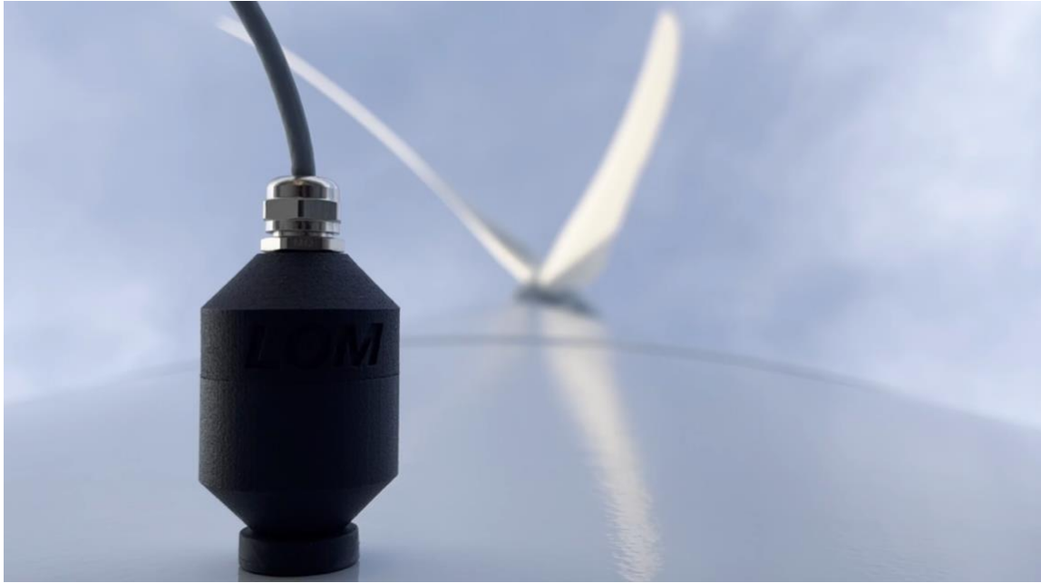
Figure 26 Geophone picking up vibrations from inside the turbine T9, Havøygavlen, Ávvá (Renzi 2023).
