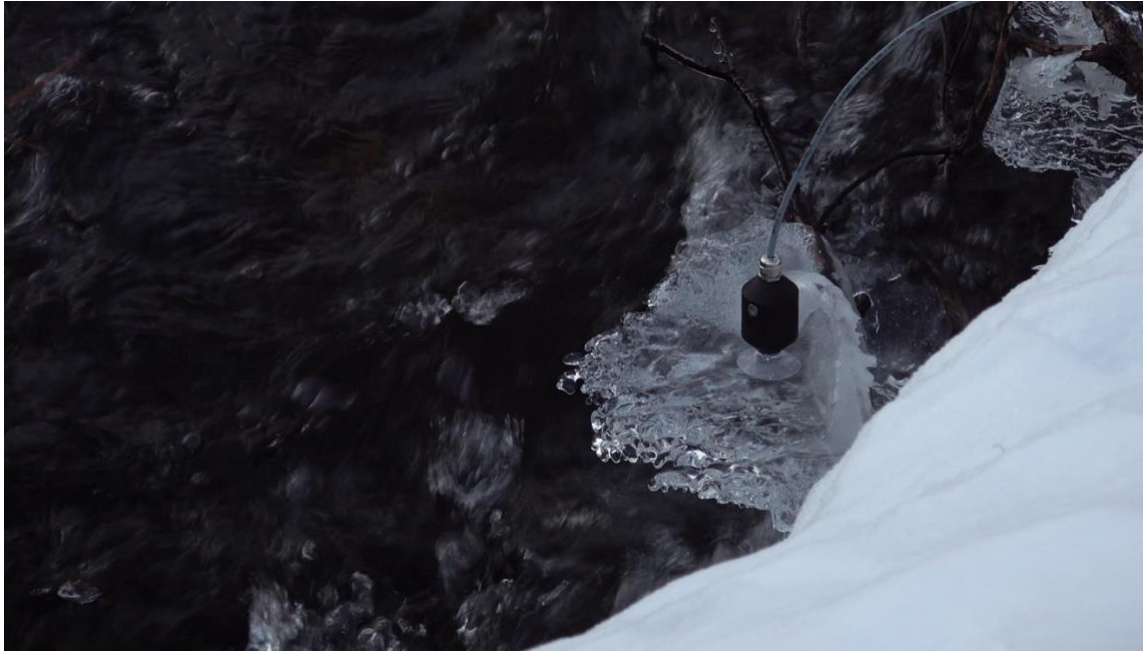
Figure 15 Geophone recording of water running under thin ice at Vuorašjohka, Ávzi ( Renzi 2023).
