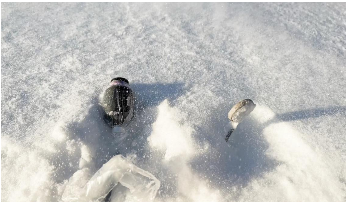
Figure 16 Geophone and contact recording of snow being windswept on frosty ground in Guovdageaidnu (Renzi 2023).
