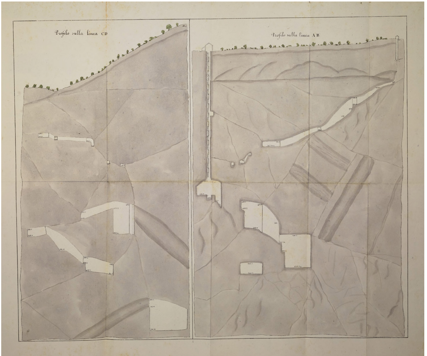
Fig. 5 - Geometry (vertical cross-section) of the underground works of the of the Lungro salt mine; survey performed in 1824 (Galli, 1828).
