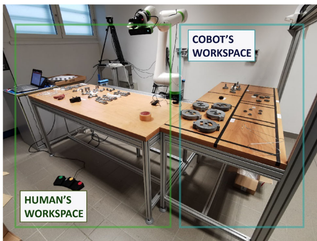
Fig. 1 Lab setting where participants performed the pick and place task with the collaborative robot
