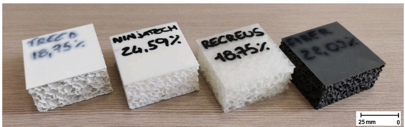
Fig. 2. Example of specimens (from left to right): Treed ElastoA (18,75%), Ninjatek Cheetah (24,59%), Filaflex Recreus 82 A (18,75%), Fiberlogy Fiberflex (28,03%).
