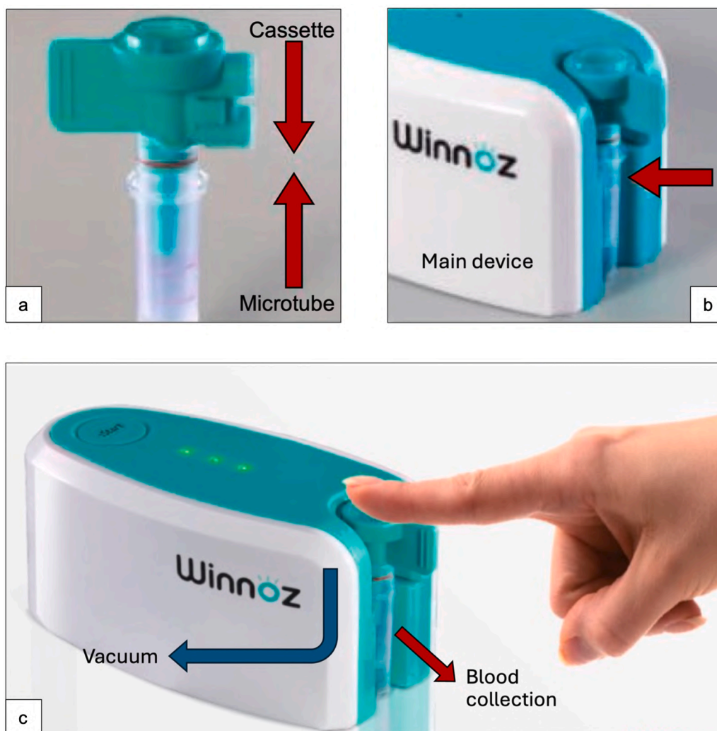
Fig. 8. Setup and use of the Winnoz Haiim Vacuum-assisted fingertip fluid blood collection: (a) insertion of the disposable cassette into an anticoagulant-treated microtube, (b) connection of the cassette to the main device and (c) process of fingertip fluid blood collection. Adapted from www.winnoz.com .
