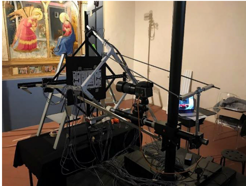
Fig. 11. The operations during the acquisition: A custom stand was developed to host cameras and lights perpendicular to the painting's plane, with eight different lights directions and a movable structure to capture the artwork's details at the desired resolution (image by G. Bacci).
