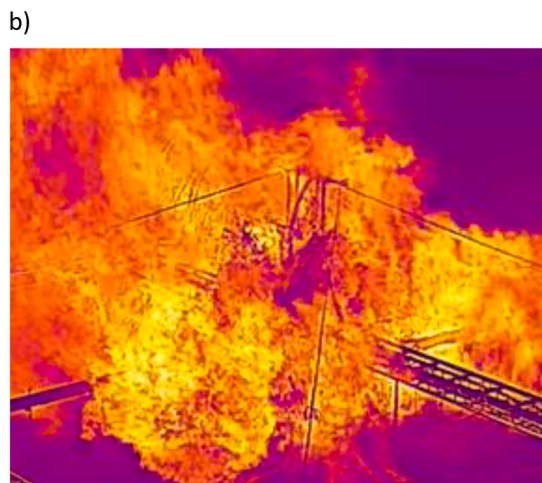
Fig. 7. View of the second LH 2 release of Trial 014: (a) the heterogeneous evaporation of the release at the basin; (b) the thermal camera frame capturing the ignited released gas cloud with fire spreading in quadrant Q3.
