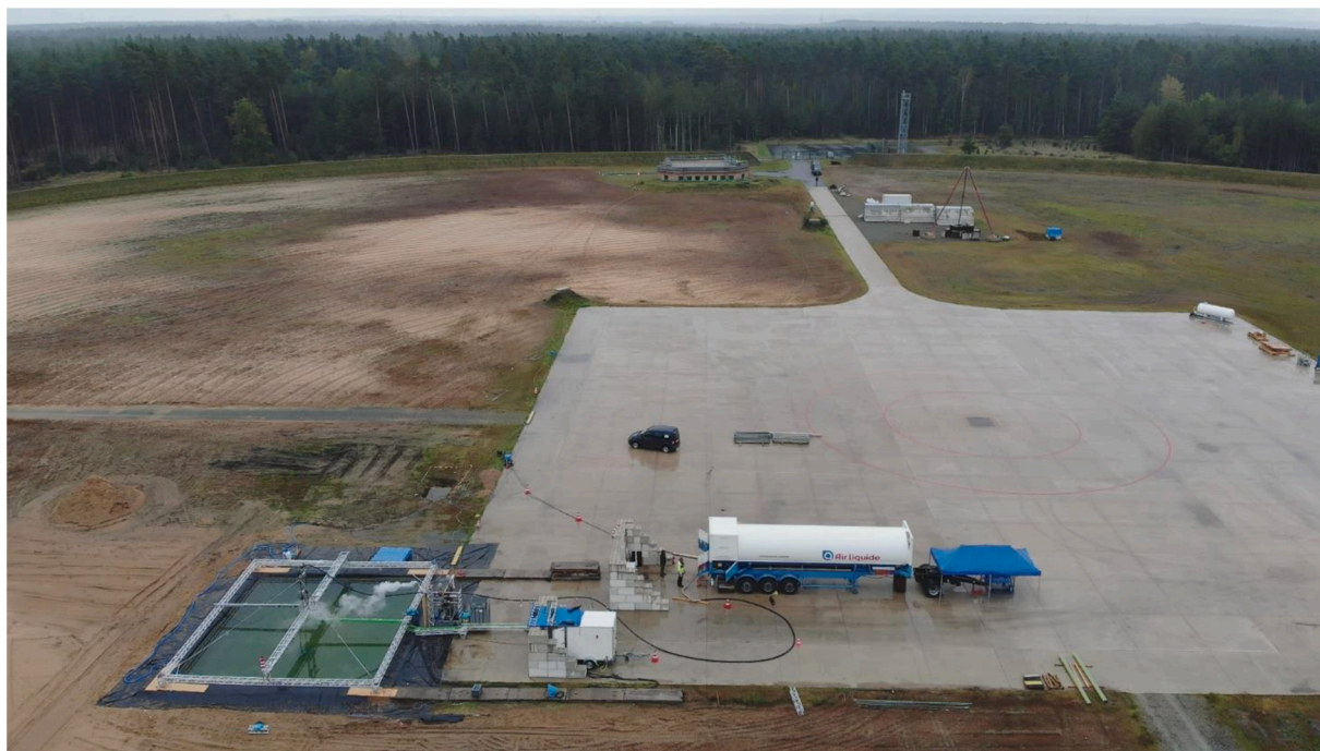
Fig. 1. Experimental test set-up at the Test Site Technical Safety of BAM to investigate LH 2 releases above and underwater. From left to right, the water basin equipped with the release mechanism and instrumentation, a cabin adapted for logging equipment, and the LH 2 delivery truck.
