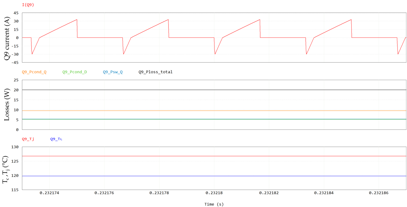
Figure 22. Q9 losses at V_{out} = 250 V and P_{out} = 4.125 kW: Q9 current, conduction losses (in orange), third-quadrant losses (in green), switching losses (in light blue), total losses (in black) and case and junction temperatures.
