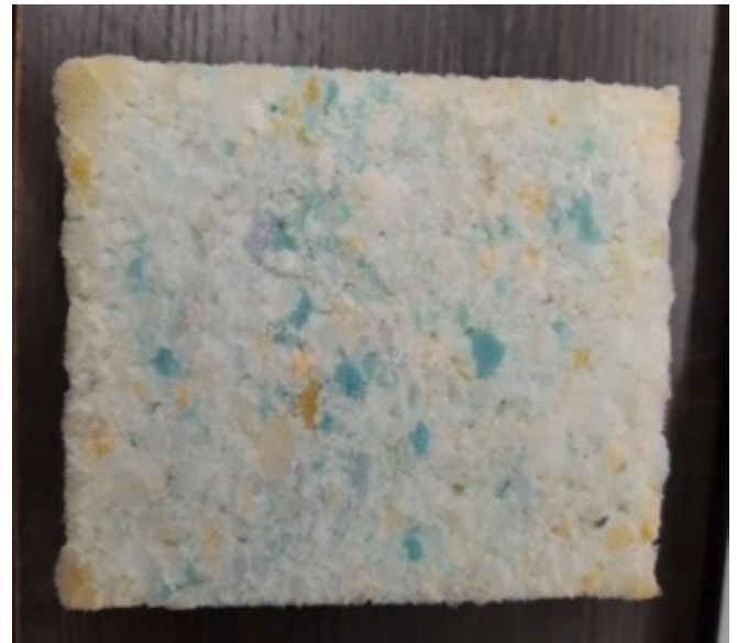
Fig. 7. Foam obtained by rebonding process of pre-consumer foam waste.
