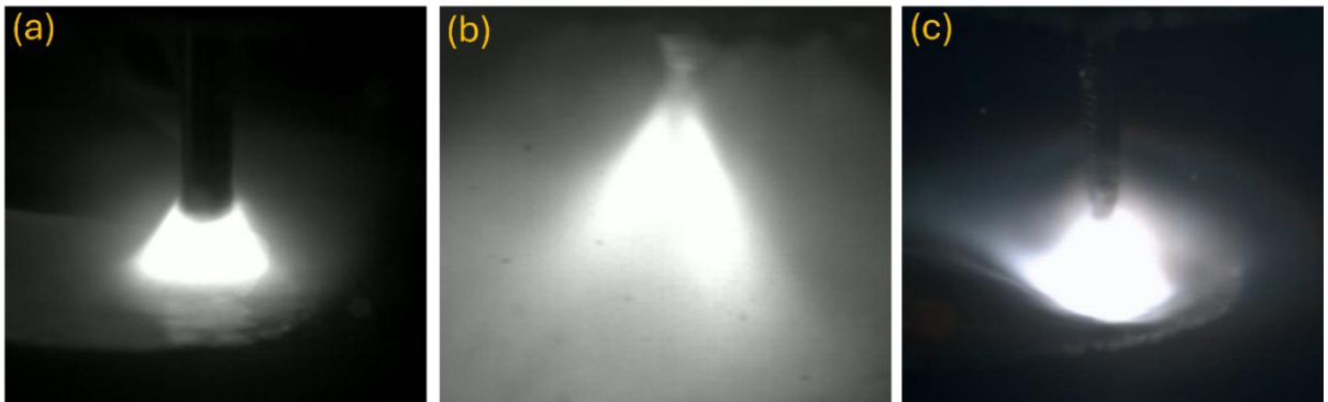
Fig. 3 Effects of shielding gases on arc stability under (a) \text{ArCO}_2 , (b) \text{ArCO}_2\text{O}_2 , and (c) Pure Argon
