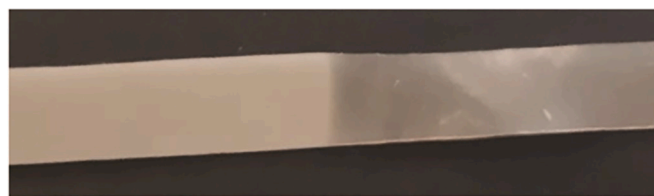
Fig. 8. Difference in transparency between the non-stretched (left) and stretched (right) area of a 2,4-PHF sample, 1 min after stretching the sample until break.
