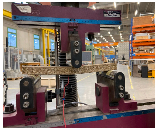
Fig. 5. Three-point bending test on a sample of 300 × 50 × 22 mm.
